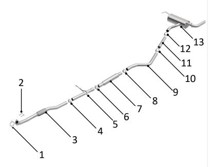
**STEP 1:** (Carefully read all instructions before installation) Disconnect the vehicle's battery before removal of the OEM exhaust system. This will prevent electrical accidents and will reset the computer if it applies to the vehicle. Remove existing exhaust system from the vehicle. Only remove parts that will be replaced. Clean existing flange with a wire brush to ensure proper sealing.
